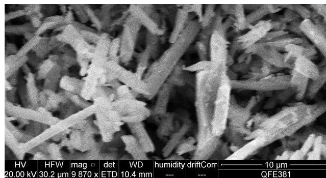
Figure 6. SEM/EDX image of the nanocrystals [\text{CuCl}(\text{Se}_2\text{Ph}_2)_2]_n formed by the reaction of [\text{C}_2\text{mim}][\text{CuCl}_2] , \text{Ph}_2\text{Se}_2 , and [\text{C}_2\text{mim}][\text{InCl}_4] (3b).
